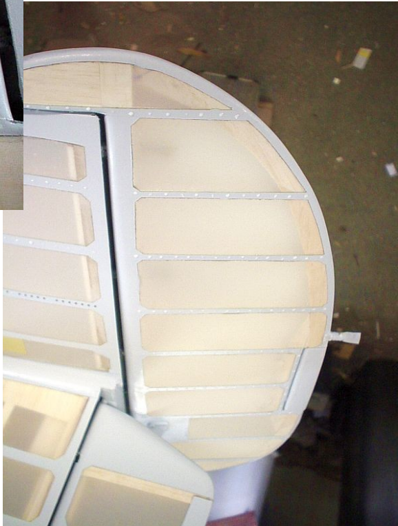
PVA rib stitching simulated on tailplane.
